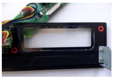
Fit the two red washers (if fitted on your unit), align the new bracket/display assembly and fix with the two (longer) screws.
