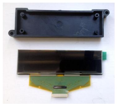
When handling the new OLED take care not to touch the silver contacts on the display flexi cable (shown at the bottom of the photo). These are static sensitive and grease from your fingers can affect the contact material. Also the OLED is made of a thin piece of glass which is reasonably fragile.
