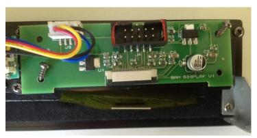
Remove the two screws holding the circuit board to the plastic bracket, remove the circuit board and release the display flexi cable.
