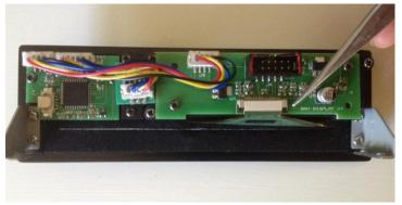
The OLED display has a flexi-ribbon cable which is held in place by a sliding retaining clip (indicated in the photo). Carefully push each side of the retaining clip towards the edge of the circuit board
