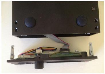
Connect the grey ribbon cable to the rear of the display panel. It will only fit one way round.
