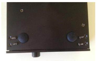
Push the front panel up to the case, so there is no gap between the front panel and the case, before tightening the four retaining screws.
