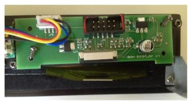
Position the circuit board and fit the two screws that hold it to the plastic bracket.
