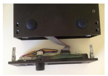
Slide the front panel forward far enough to disconnect the grey ribbon cable from the Display panel.
