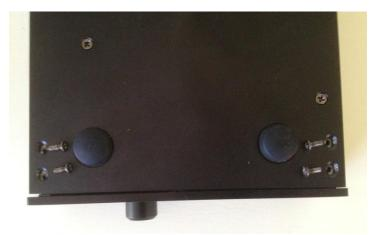
Turn the B2 over and remove the four screws as shown in the photo above.
